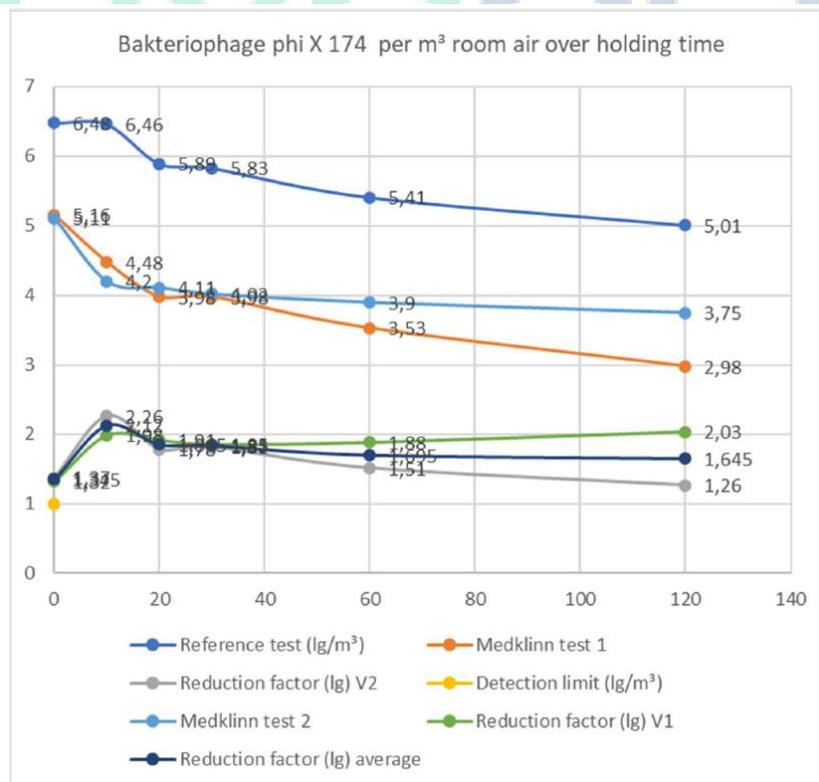
After 10min the maximum reduction factor was measured as a 2.12lg reduction (99% reduction) compared to the reference test, when the Medklinn PRO AS2 Air+Surface
